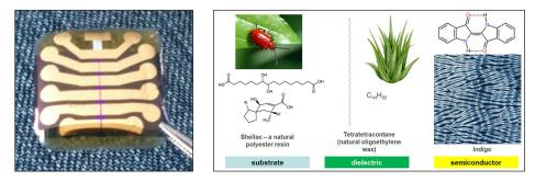
An example of thin-film indigo transistors fabricated from natural materials. A photo of the finished devices is shown on the left, while the schematic of materials from substrate, dielectric, to semiconductor is shown on the right.
